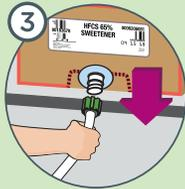
Remove connector and replace with new HFCS sweetener BIB.
