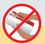
po NOT physically separate double cartridges before inserting into plastic trays. If cartridges are separated, the dispenser will not prime the cartridge. Call service at 800.241.COKE to flush lines.
