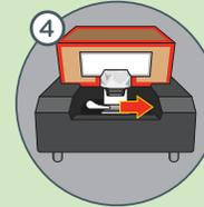
Place box onto tray with the arrows on the package facing up. Align fitment to connector, then move lever to the right to lock.
