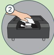
Remove collar. Clean collar, probe and compartment with cloth dipped in approved sanitizer. Wait 2 minutes and repeat with fresh sanitizer then allow to air dry.
