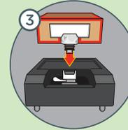
Reinstall the collar. Open the new box, pull out the fitment and remove cap. CAUTION: Do not use a sharp object to open
