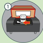
Release by moving locking lever to the left. Double check to ensure the box is empty and remove.
