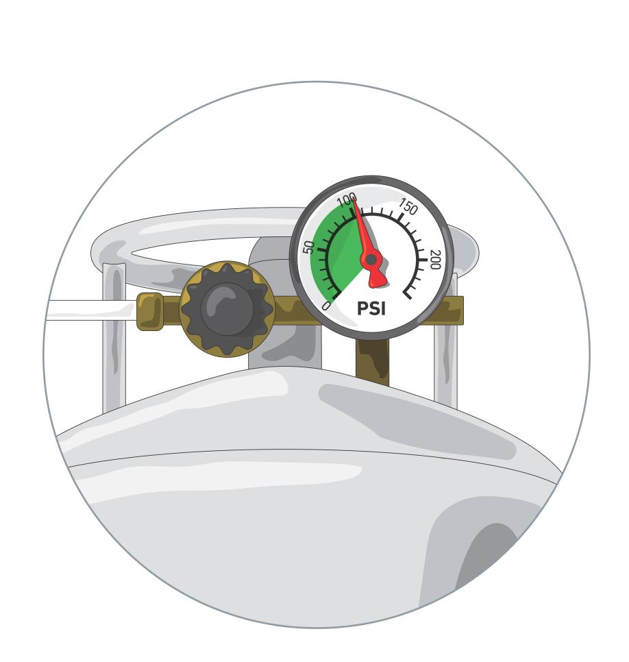
Is the CO<sub>2</sub> pressure gauge higher than 100PSI?
