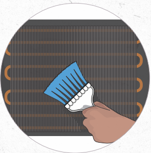
3 Clean condenser fins with the condenser brush
