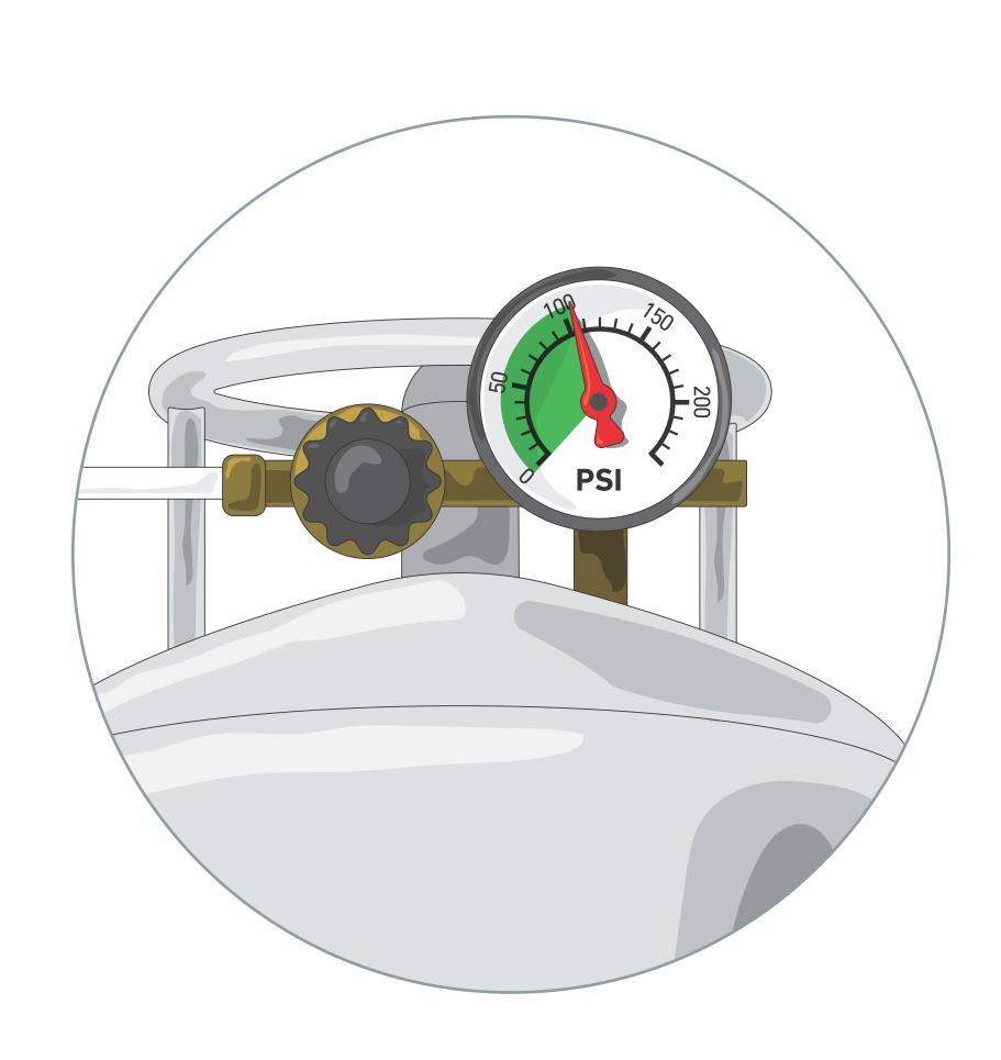
Is the CO<sub>2</sub> pressure gauge higher than 100PSI? IF NO, call your CO<sub>2</sub> service provider.
