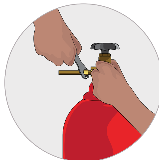
Loosen the connection nut
