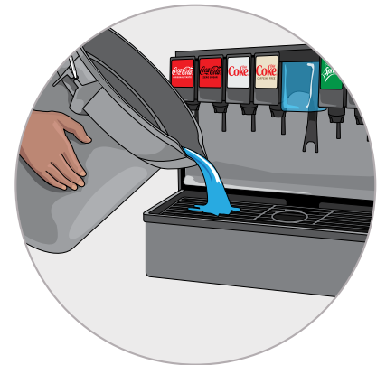
Pour chlorine-based sanitizer solution over the cup rest
