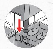
Place o-rings on dispense valves (check to see if nicked or twisted) and place valve in bowls.
