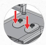
Install mixing impellers.
