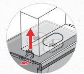
Press release latch on front of the machine before removing bowls.
