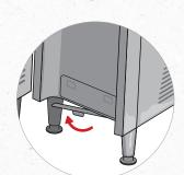
Rotate support brackets for drip tray.
