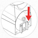
Install auger nose bushing into interior slots.
