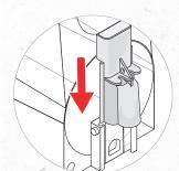
Carefully slide faucet valve assembly into place on the hopper.
