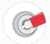
Apply lubricant to grommets on side facing cooling drum.
