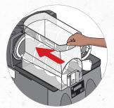
Install hoppers over the augers and cooling drums.
