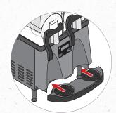
Assemble drip tray and slide onto metal extensions from base.
