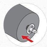
Install grommets (push as far as they will go) on the ends of the cooling drums.
