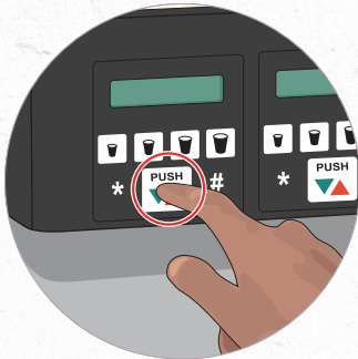
4 Press the PUSH button to flush each valve until only clear water is dispensed.
