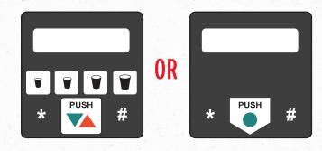
Navigate the service menu by pressing the \* and # buttons to scroll up or down the list. Press the PUSH button to accept the current selection. When presented with a Yes/No option, press \* for No and # for Yes.
