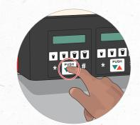
Press the PUSH button to dispense a small amount from each valve until product is visible
