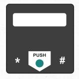
Navigate the service menu by pressing the and buttons to scroll up or down the list. Press the PUSH button to accept the current selection. When presented with a Yes/No option, press for No and for Yes.
