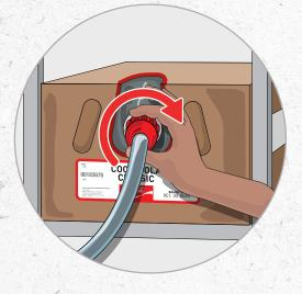
Reconnect to the correct Bag-in-Box. Tighten until the connectors are fully engaged.
