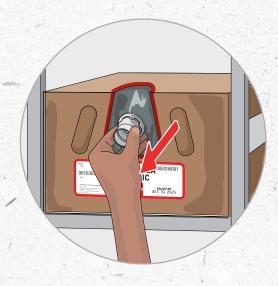
Pull the bag connector through the opening and remove the plastic dust cap.
