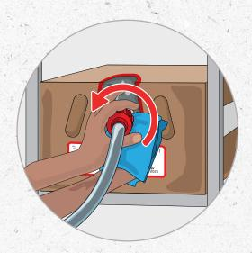
2 Unscrew the syrup line connector and remove the empty box.
